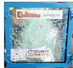
Safety2u Test Standard for Film & Glass 9mm - AS INZS 2343 - 1997 (GO)
